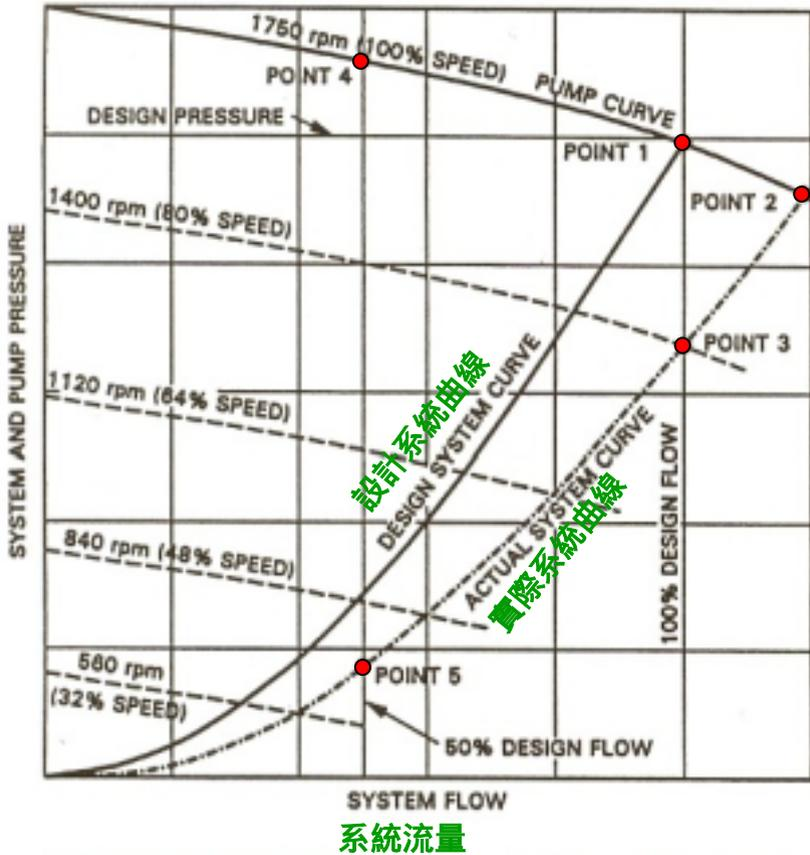
FIGURE 4-16 Variable Speed Pump Operation
